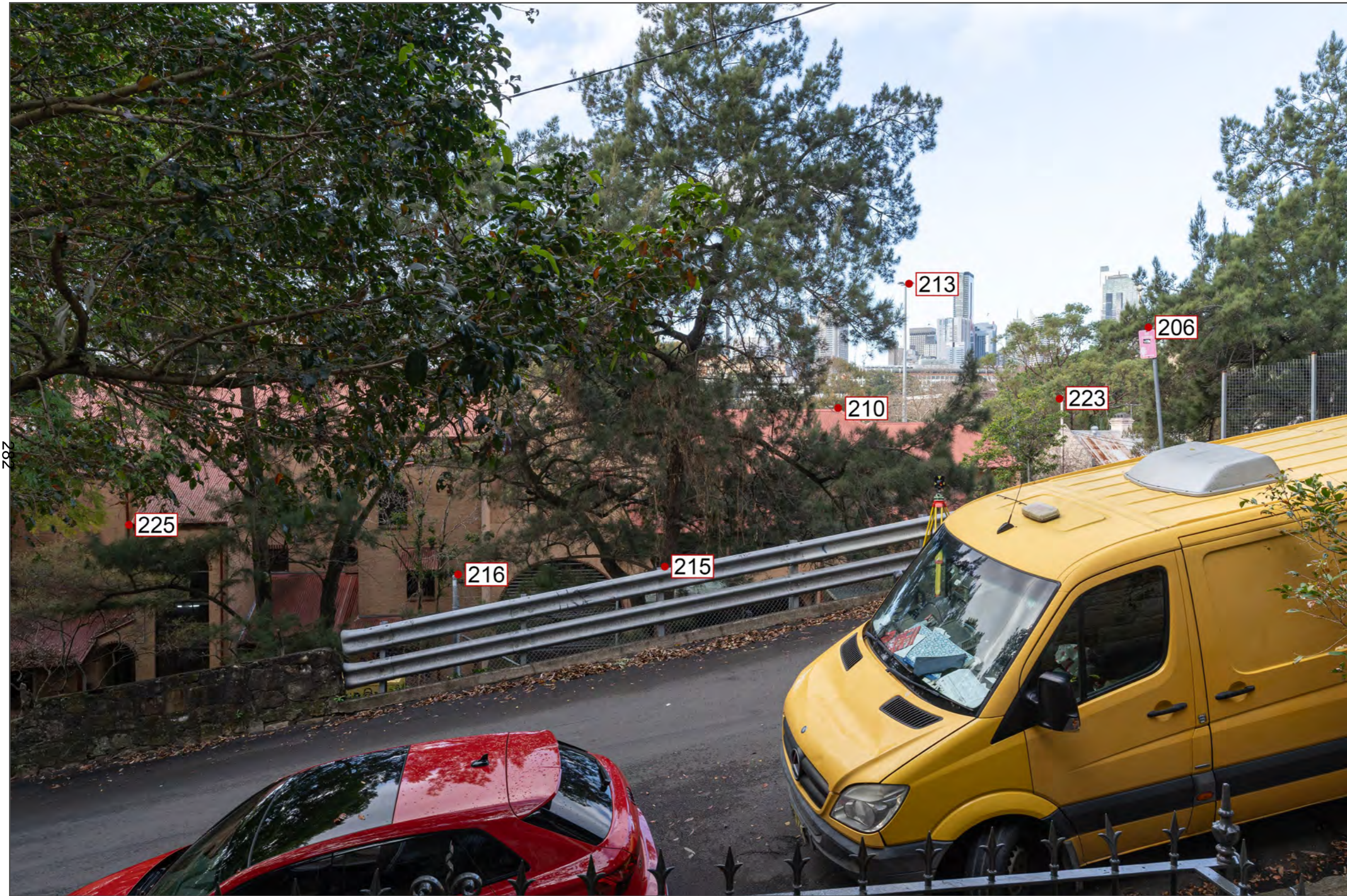
OVERLAY OF SURVEY POINTS USED FOR 3D CAMERA ALIGNMENT
